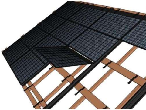
Fig. 6 Placement of the solar panel
